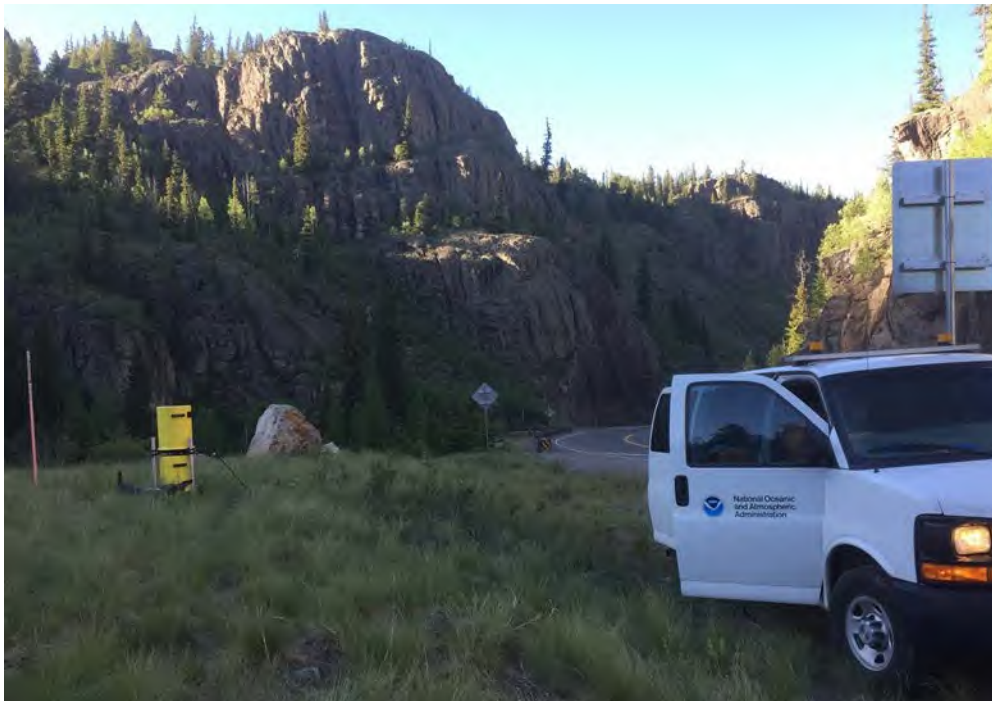
Figure 7: A10 Absolute Gravimeter deployed in the field
